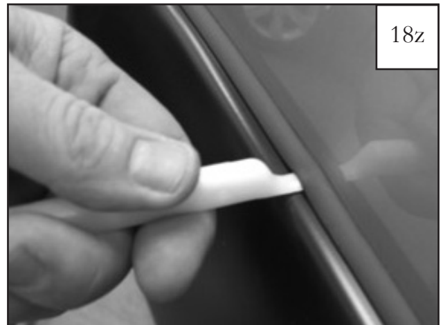
18z Using flat end of supplied Edge Trim Tool (ET1-0002), seat edge trim against flare by inserting straight end between edge trim and flare at one end. Next, slide around entire edge to the other end.
