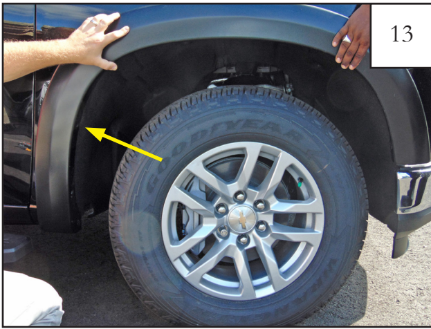
13 Install (1) supplied phillips head screw (SW1-0058) at rear Clip location. Do not tighten. (If needed use an awl to align flare mounting holes.)
