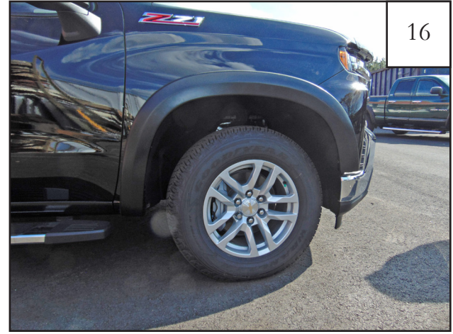
16 Completed front flare installation.
