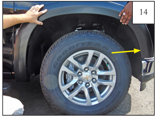
14 Install (1) supplied phillips head screw (SW1-0049) at front Clip location. Do not tighten. (If needed use an awl to align flare mounting holes.)
