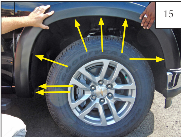
15 Press flare firmly against body and tighten all screws.
