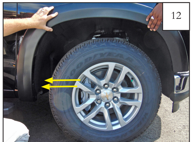
12 Re-install (2) factory screws (removed in Step 2) with a T15 bit. Do not tighten.
