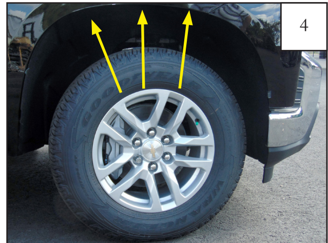
Remove (3) factory installed T15 screws from wheel well as shown above. These screws will be re-used to install the front flare.
